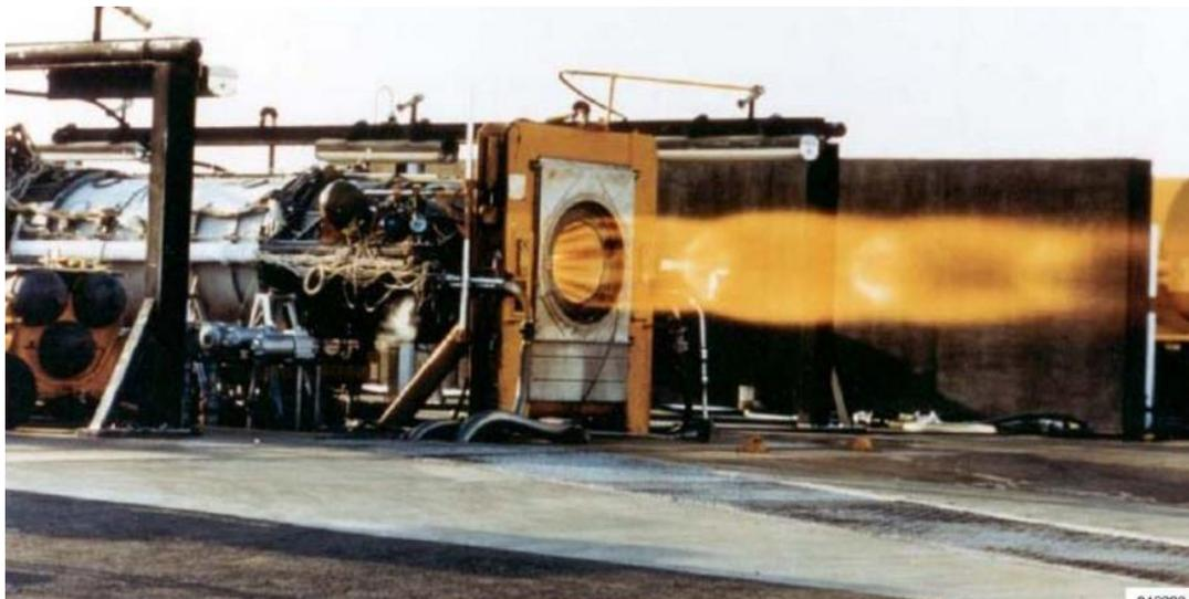
Some typical rocket emission factors are provided by AP-42; however this is not all the rockets that are tested at Air Force installations. Most commonly, if rocket motor testing is conducted there are specific emission factors and test data that provide a more accurate emission profile. It is suggested to use the more accurate data than the factors provided in AP-42.
