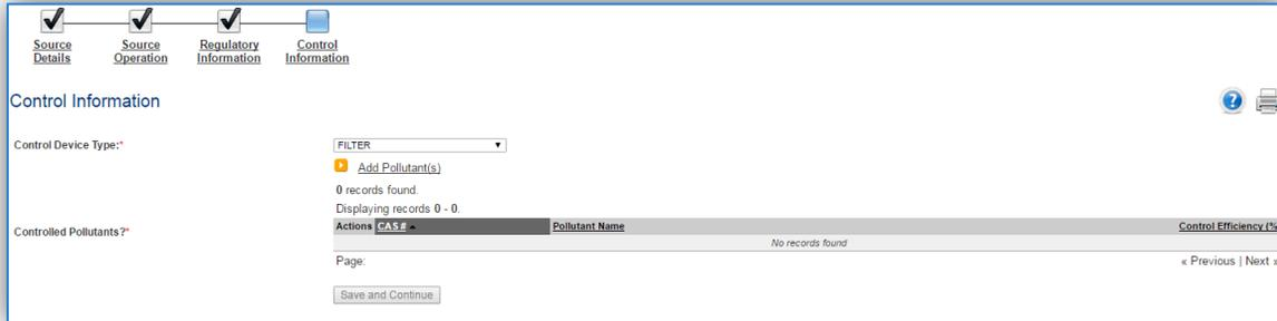
Select **Control Device Type** utilized by the equipment: BAGHOUSE, CYCLONE, DRAPE, DUST ENCLOSURE, ELECTROSTATIC PRECIPITATOR, FILTER, VACUUM BLASTER, WATER CURTAIN or WET BLASTING.
